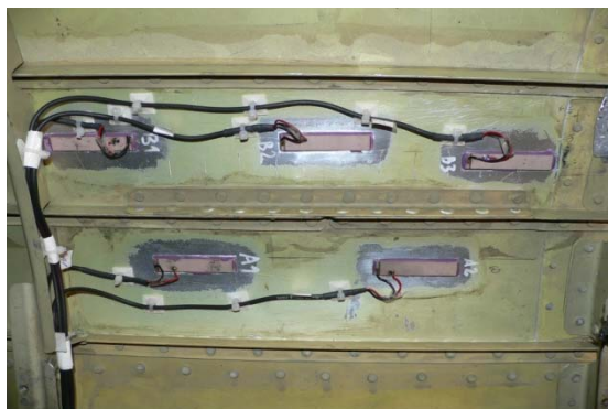
Sensors location in a zone between 7 th and 8 th frames (inner view)
