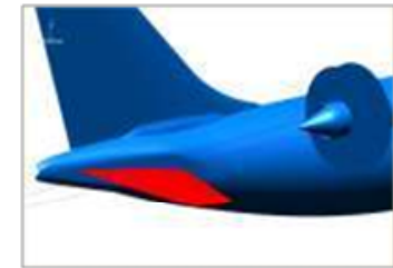
CROR design study: interference with HTP
